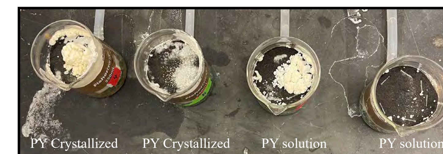
Figure 13 : Indicates positive trend of efflorescence when Prussian yellow and capillary mats are utilized
